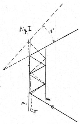
angle that the mirror is turned. The magnification is increased by increasing the number of reflections and by turning both mirrors in opposite sense. It is evident that in Figure I if the short mirror had turned an equal amount in the opposite sense to the long mirror, we would have increased our magnification.
