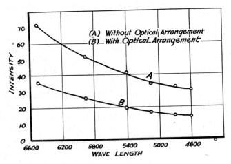
From the curves it will be seen that there is a gradual, almost continuous decrease from 50 per cent to 45.16 per cent in the intensity transmitted, as we pass from the longer to the shorter wave lengths of the spectrum.
