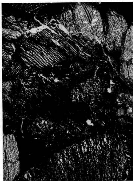
Fig. 3 (above).—Coal particles 35 x 48 mesh; a. fusain; b. vitrain
