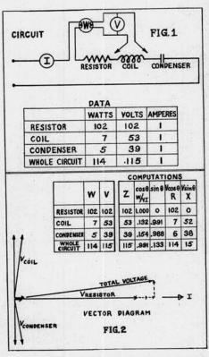
If desired these data can also be used to analyze the impedence of L and C into reactance and resistance, so that the inductance and capacitance and power factors can be computed.
