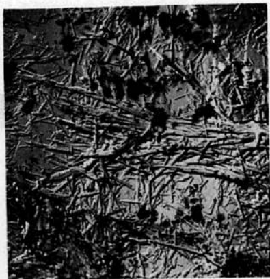
FIG. 8.—Electron micrograph of fracture surface of virtually undolomitized Platteville limestone, showing acicular crystals, probably sepiolite. Magnification approx. X 2,000.
