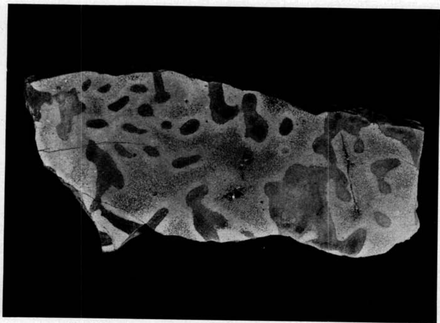
FIG. 5.—Ground, etched and stained "fucoidal" dolomite. Magnification approx. X 0.7.
